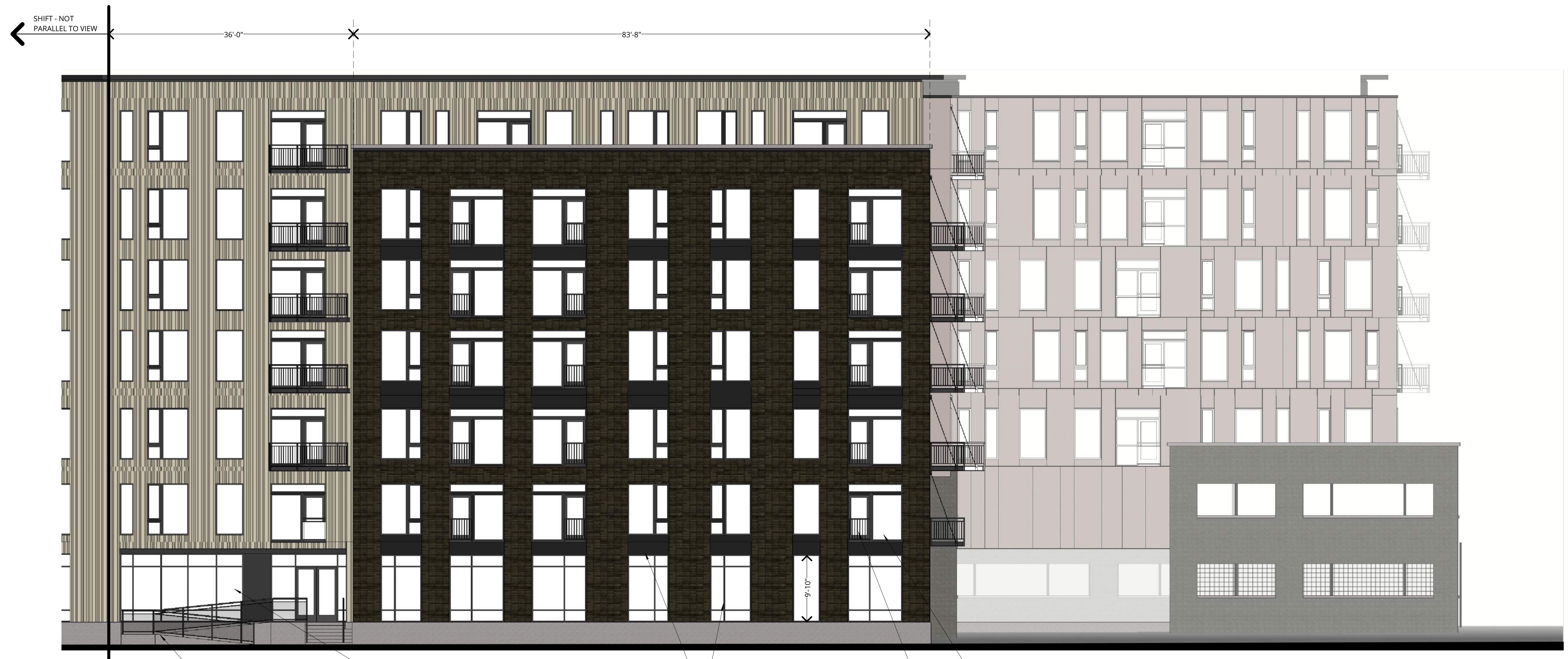
NORTH ELEVATION - WEST SIDE 1/8" = 1'-0" 0 4 8 16 32 CONCRETE RAMP W/ BLACK T.S. GUARDRAIL W/ WELDED WIRE MESH INFILL PANELS RECESSED STOREFRONT ENTRY @ LOBBY BLACK METAL 2x6 STOREFRONT - CENTER SET GLAZING SMOOTH BLACK METAL INFILL PANEL - GAUGE T.B.D. TO PREVENT OIL CANNING VINYL WINDOW - ECO - CHARCOAL EXTERIOR COLOR INTEGRAL VERTICAL PICKET JULIET RAILING
