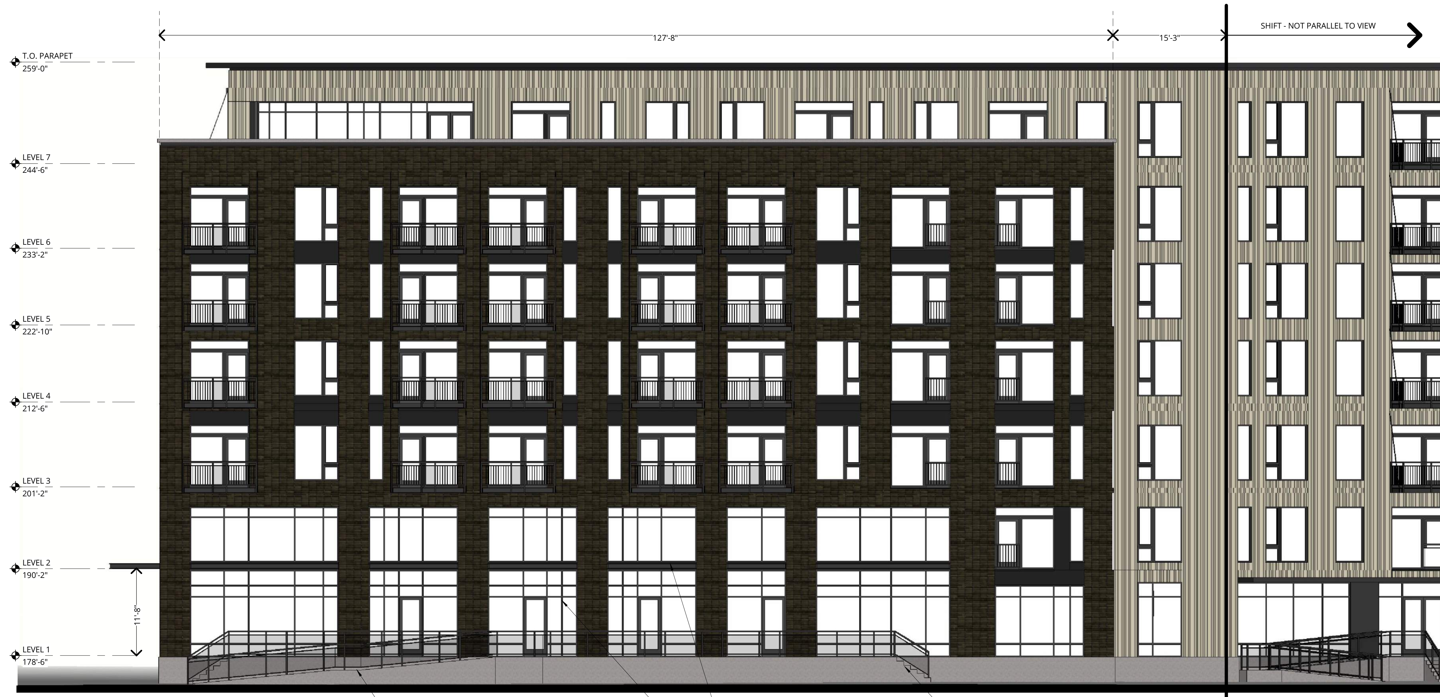
NORTH ELEVATION - EAST SIDE 1/8" = 1'-0" 0 4 8 16 32 CONCRETE RAMP W/ BLACK T.S. GUARDRAIL W/ WELDED WIRE MESH INFILL PANELS STEEL CANOPY WITH INTEGRAL LIGHTING. SHED TOWARDS FRONT. WOOD TEXTURE METAL SOFFIT. 8" CHANNEL SURROUND. CONCRETE STAIR BLACK METAL 2x6 STOREFRONT - CENTER SET GLAZING
