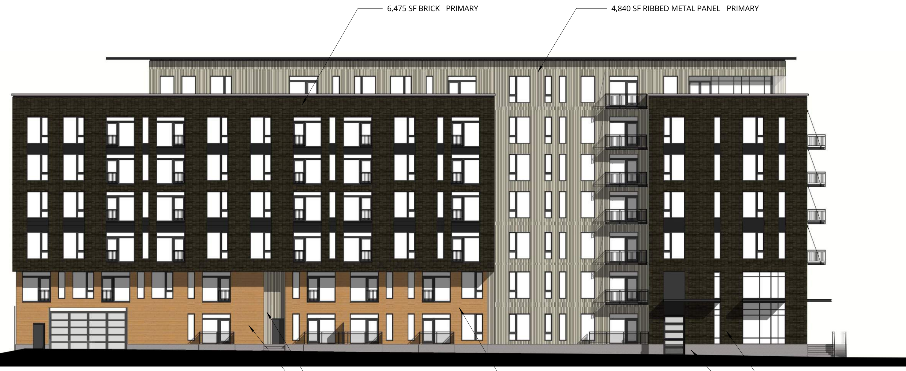
EAST ELEVATION 1/16" = 1'-0" 0 8 16 32 64 EAST ELEVATION 17,210 SF PRIMARY 100%
